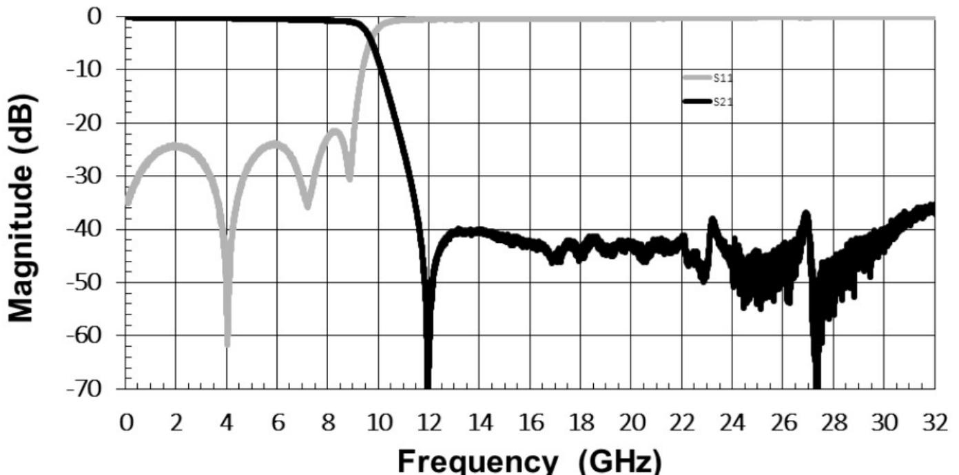
\*Typical de-embedded measured performance mounted on a connectorized test fixture. DEB is 0.254mm RO4350B with 50.0Ohm CPW ground traces going into the ports at room temperature.
