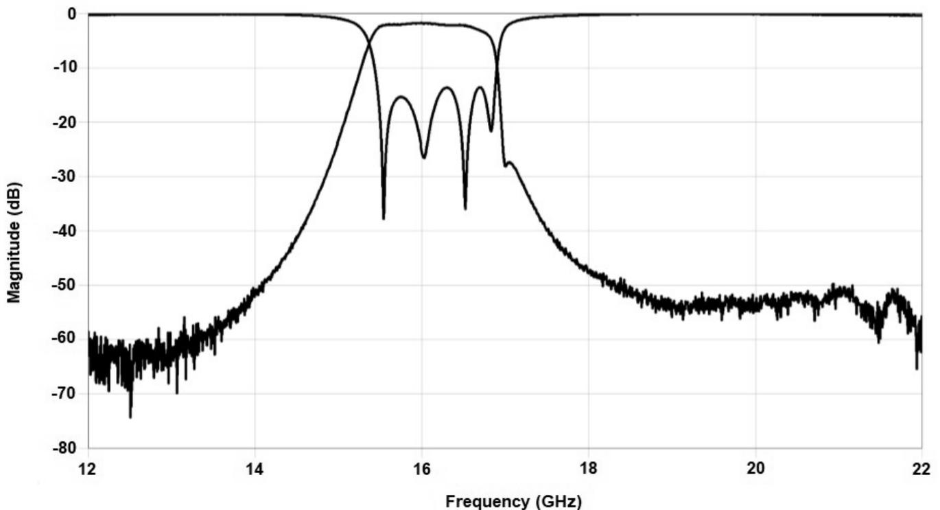
\*Typical de-embedded measured performance mounted on a connectorized test fixture. DEB is 0.254mm RO4350B with 50.0Ω CPW ground traces going into the ports at room temperature.
