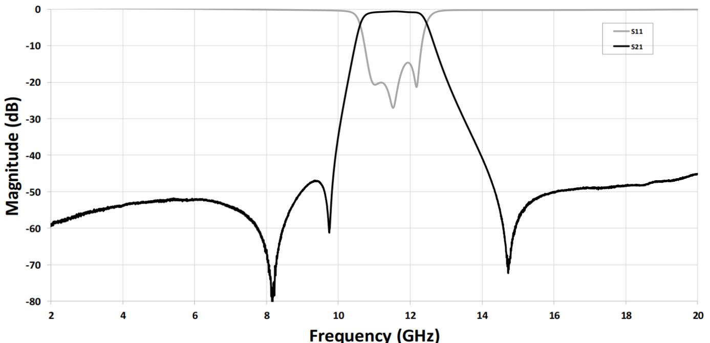
\*Typical de-embedded measured performance mounted on a connectorized test fixture. DEB is 0.254mm RO4350B with 50.0Ohm CPW ground traces going into the ports at room temperature.
