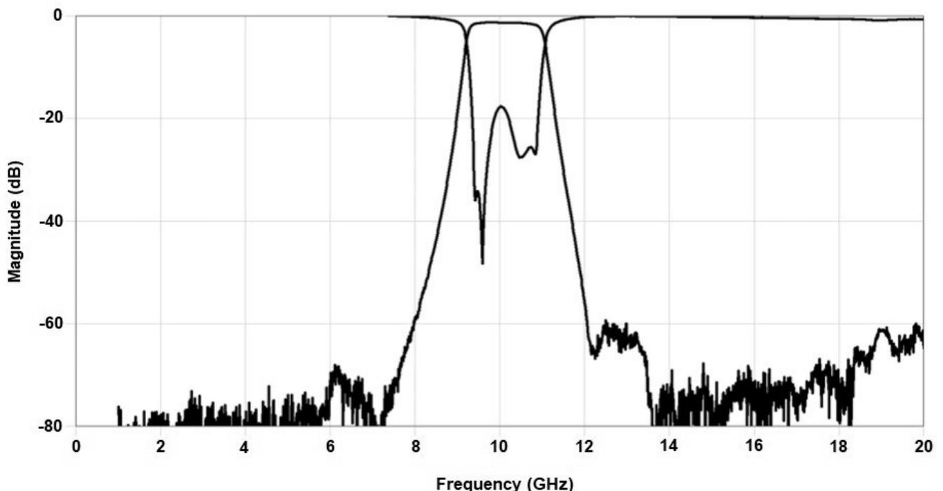
\*Typical de-embedded measured performance mounted on a connectorized test fixture. DEB is 0.254mm RO4350B with 50.00ohm CPW ground traces going into the ports at room temperature.
