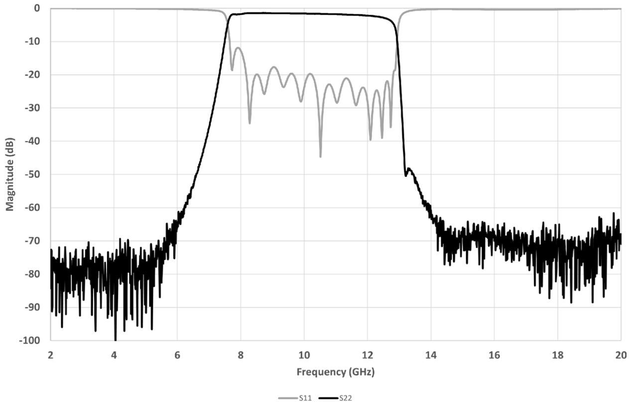
\*Typical de-embedded measured performance mounted on a connectorized test fixture. DEB is 0.254mm RO4350B with 50.00hm CPW ground traces going into the ports at room temperature.
