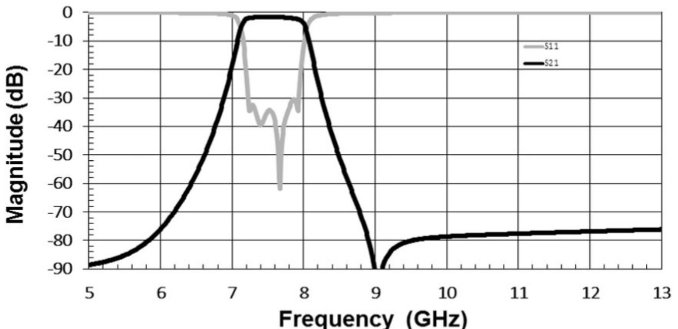
\*Typical de-embedded measured performance mounted on a connectorized test fixture. DEB is 0.254mm RO4350B with 50.0Ω CPW ground traces going into the ports at room temperature.
