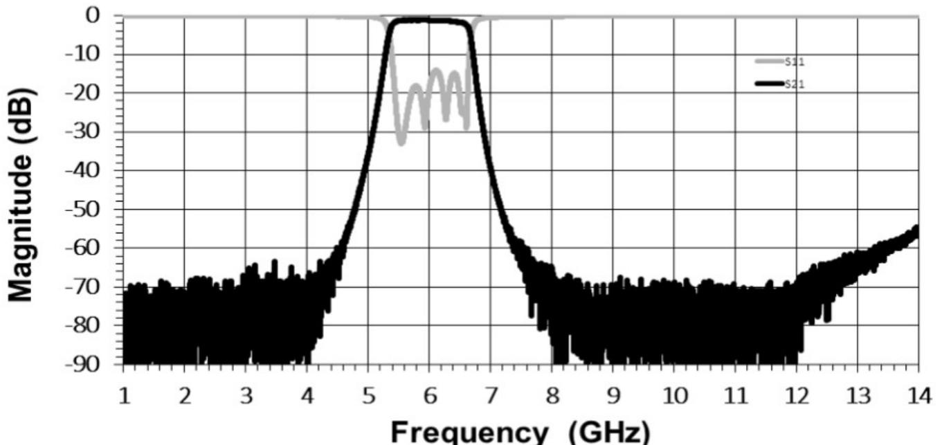
\*Typical de-embedded measured performance mounted on a connectorized test fixture. DEB is 0.254mm RO4350B with 50.0Ω CPW ground traces going into the ports at room temperature.
