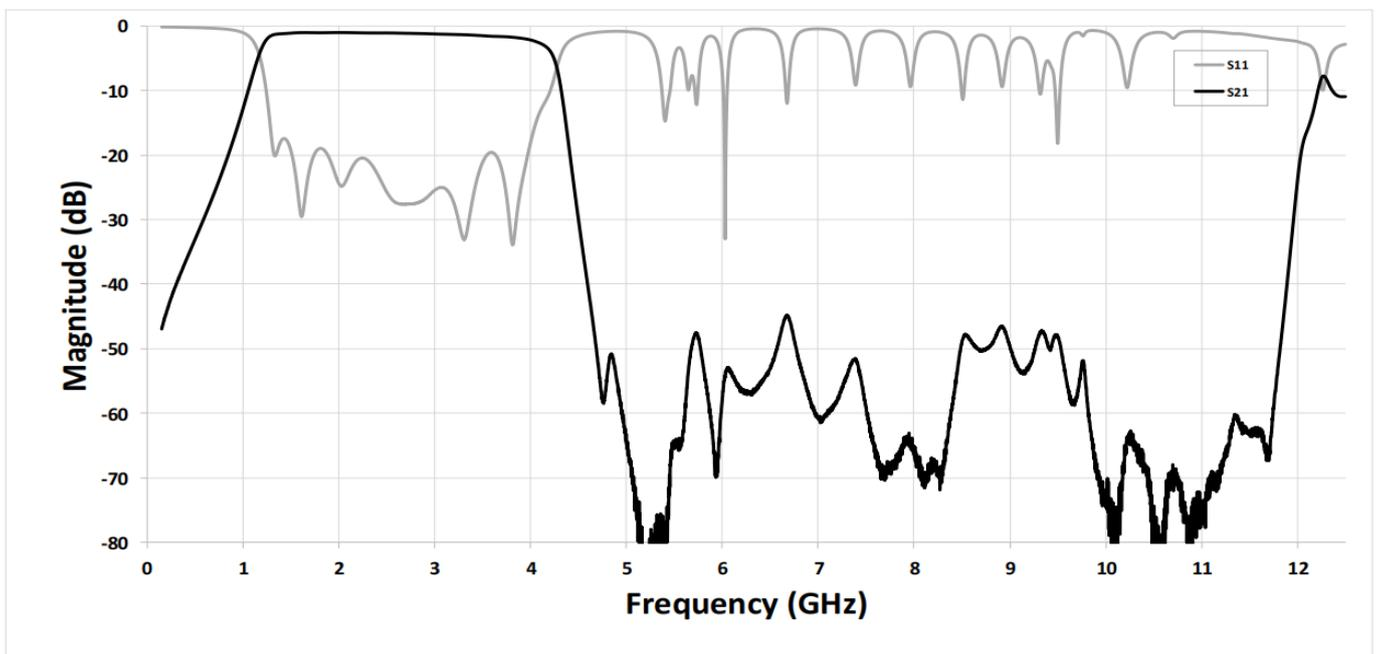
\*Typical de-embedded measured performance mounted on a connectorized test fixture. DEB is 0.254mm RO4350B with 50.00ohm CPW ground traces going into the ports at room temperature
