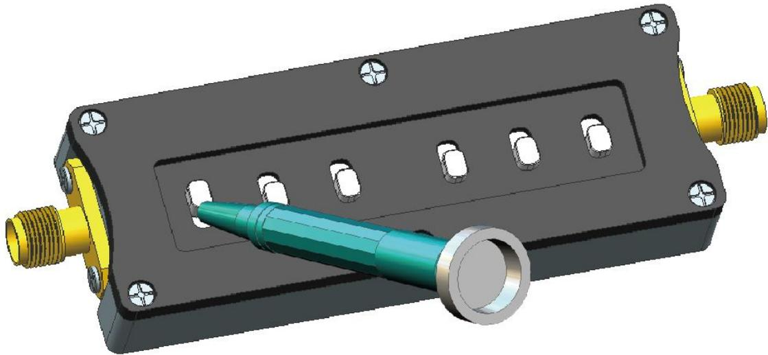
It is much easier to adjust the switch by tools like plastic screw driver.
