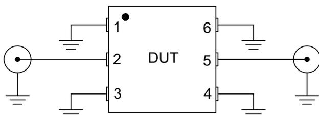
Block diagram fo Test Circuit used for characterization.
